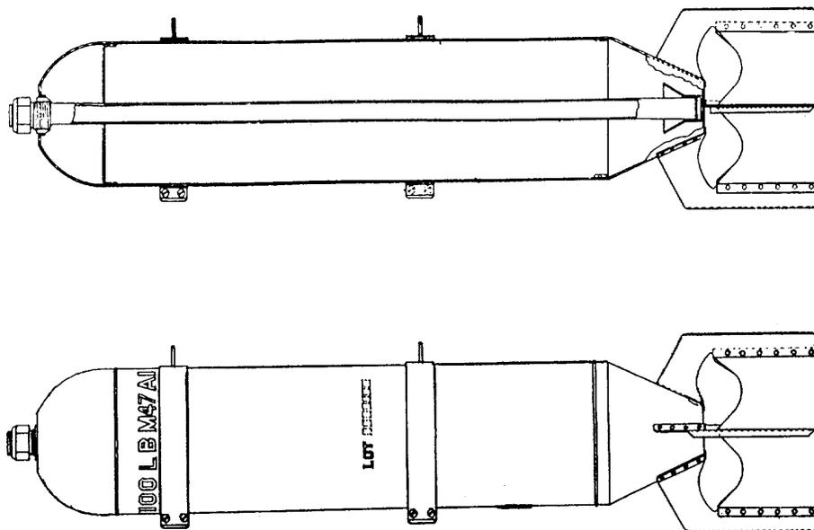
*General.* The bomb was developed to meet the requirements of the Air Forces for a chemical bomb for "bombardment" purposes. It is a thin case bomb whose design and construction is such as to provide maximum efficiency after release from the plane.
