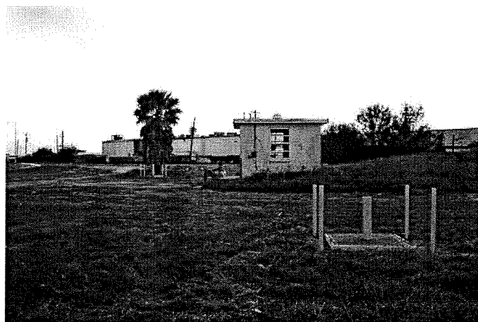
Two groundwater monitoring wells at the IWTP used for collecting groundwater samples for laboratory analysis.
