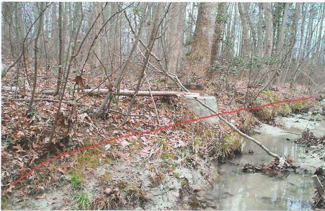
Figure 8. Looking upstream and downstream to establish bankfull stage from field indicators
