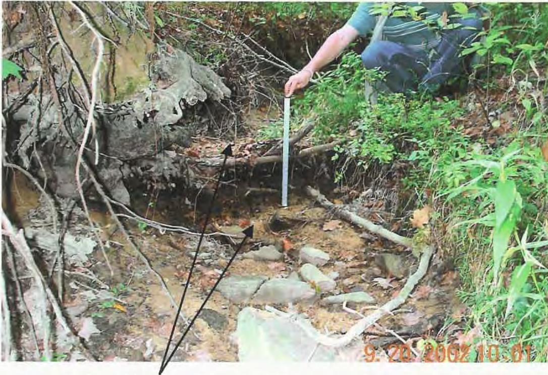
Figure 7. Channel Incision : Change in BHR due to head-cut
