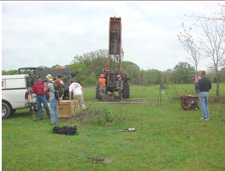
Photograph No. 1 Viewing easterly at Boring 1. Electrical restivity log equipment shown. April 7, 2005
