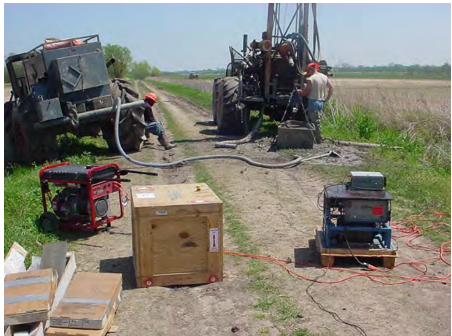
Photograph No. 2 Viewing easterly at Boring 3. Electrical restivity log equipment shown. April 9, 2005
