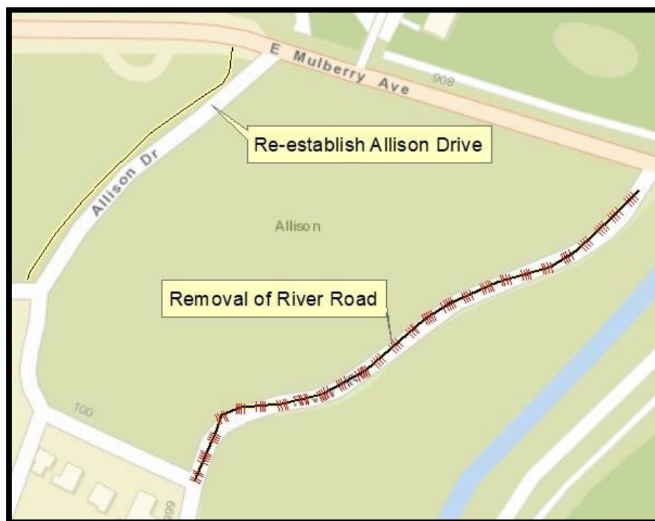
Figure 23. Re-establishment of Allison Drive
