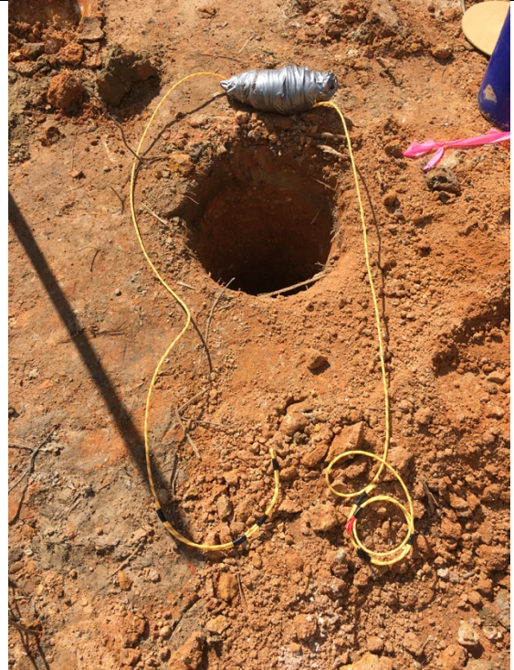
AN-M50 series incendiary pieces prepared for disposal operations
