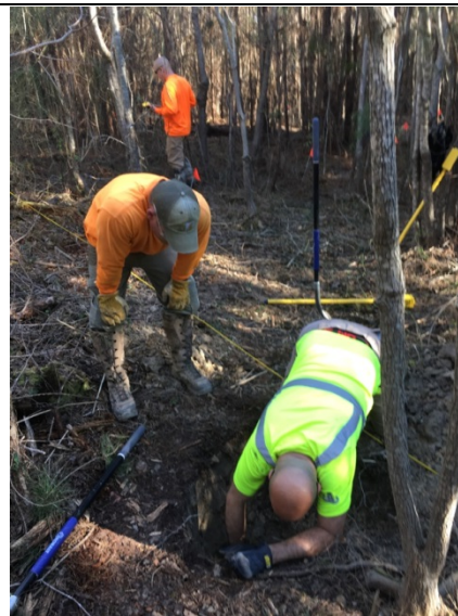
Mag and dig intrusive operations G-6
