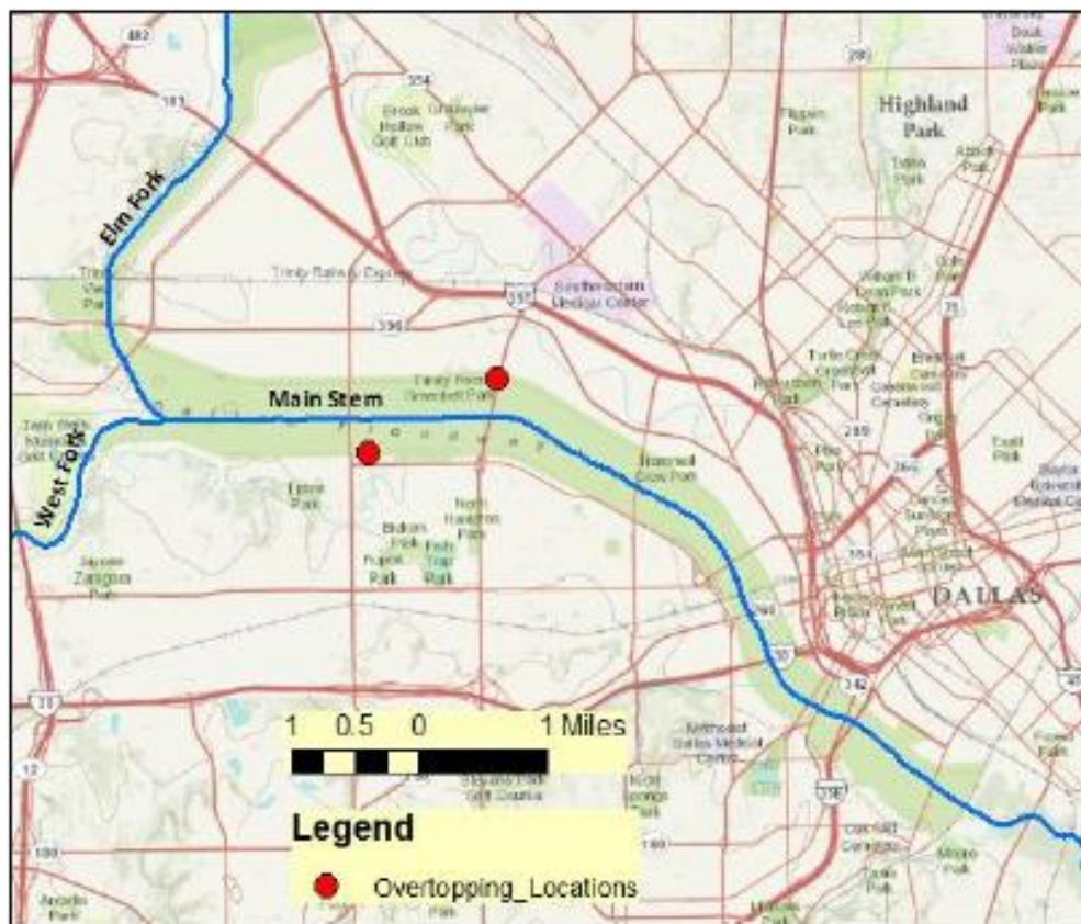
Figure 2-5 Modeled Breach Locations for Overtopping
