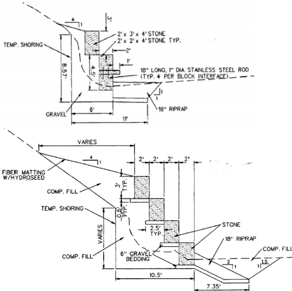
Figure 2. Typical cross sections of two types of cut stone bank stabilization
